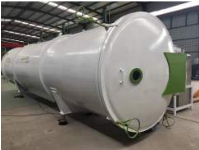
12mm thick tank wall
